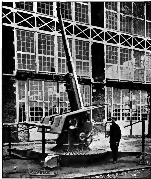
FIG. 53.—Schneider 105-mm. gun, on anti-aircraft mounting. Firing position.
