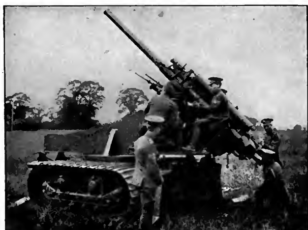
FIG. 56.—3.6-in. anti-aircraft mounting, on caterpillar truck.
