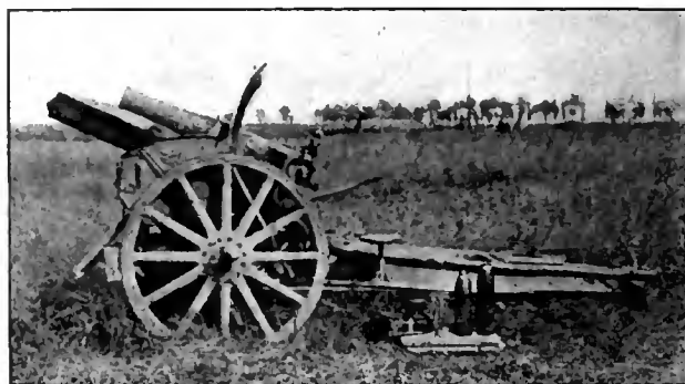
FIG. 18.—German 105-mm. field howitzer, 1898-1909.
