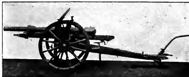
FIG. 8.—British 18-pdr. gun and carriage, 1918.
